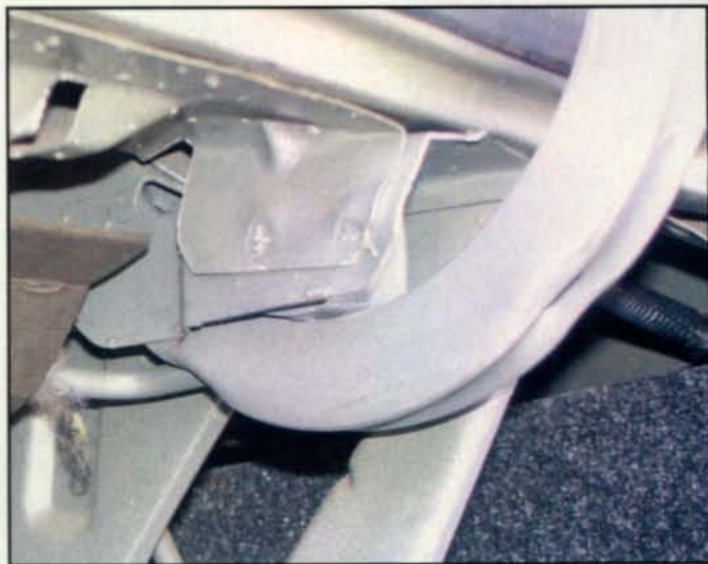
Photo B— Electrically-isolated trunk hinges.
