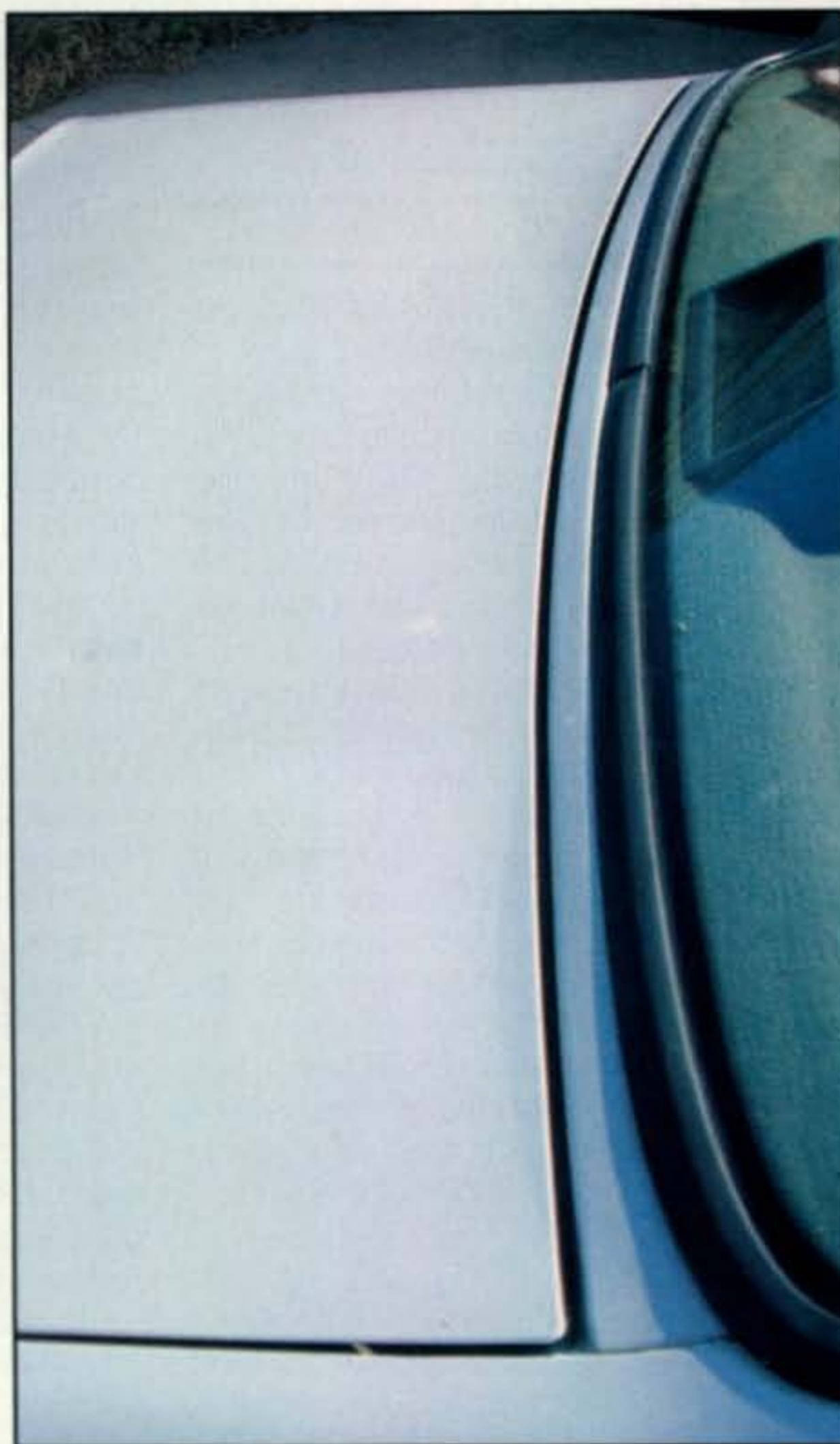
Photo C— Using parts of the vehicle as a slot antenna.
