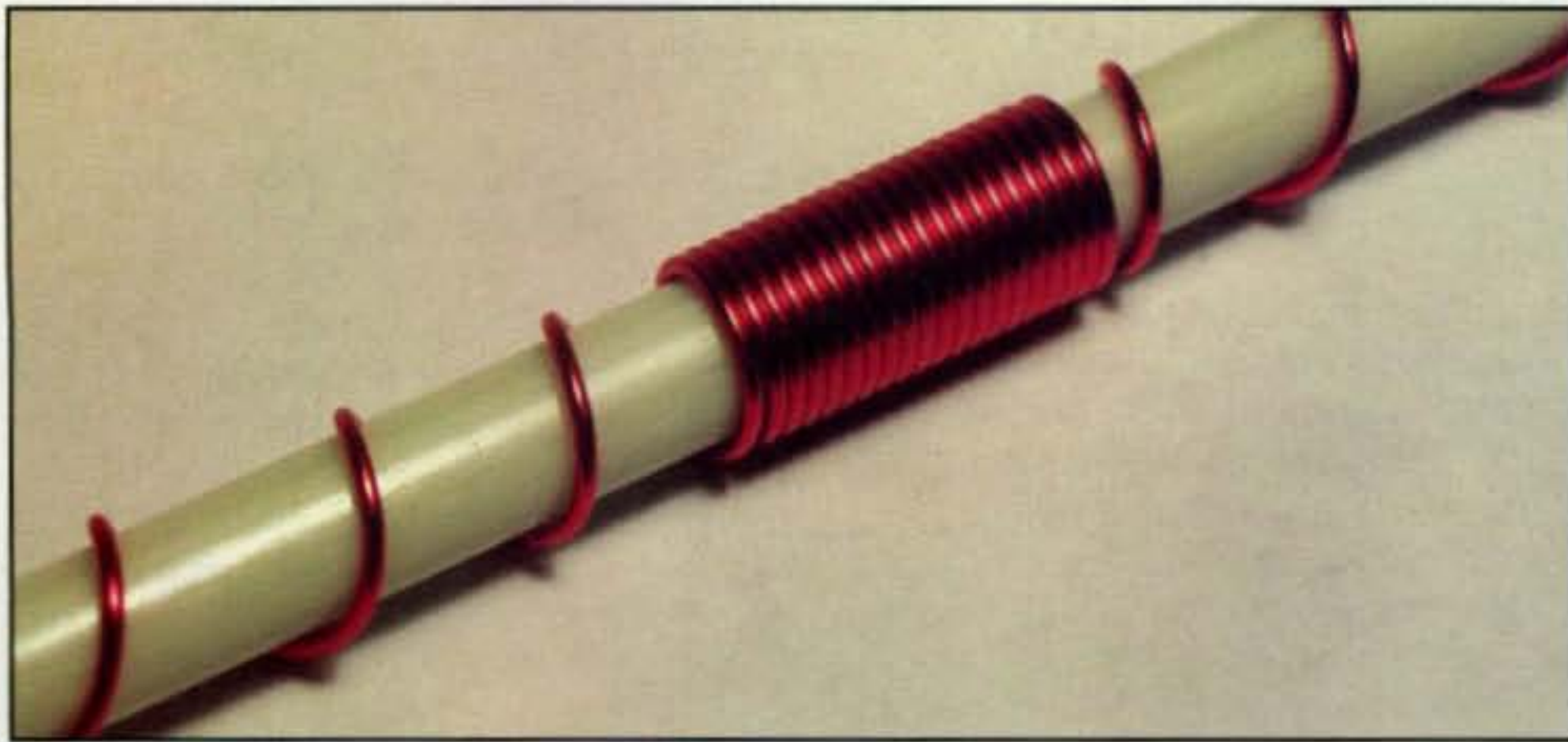
Photo E—Band-separating inductor.
